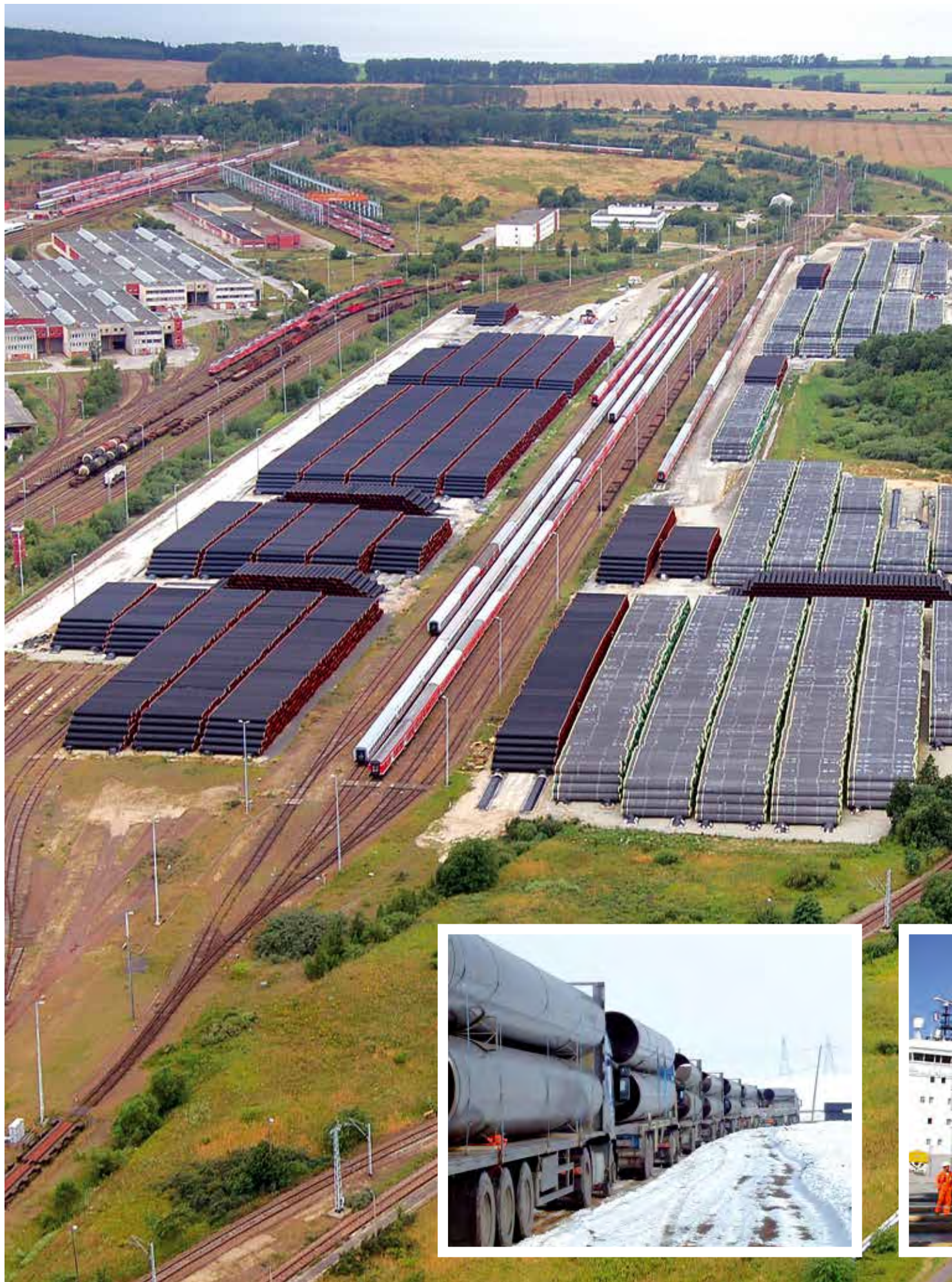
Pipe storage site at Mukran, Germany for the Nord Stream pipeline
