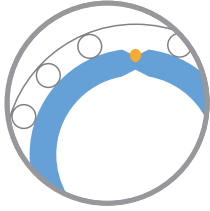
Tack welding of the slit pipe
